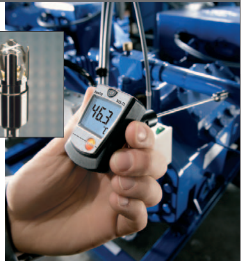
Monitoring surface temperature in refrigeration systems
