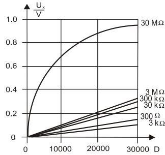
Voltage  $U_x$  across the resistance  $R_x$  to be measured as a function of measuring range and display.
