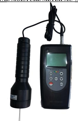
This Instrument is Digital Pin Type Cigarette Moisture Meter with Automatic Calibration Function Suitable for any Material Moisture Measurement.
